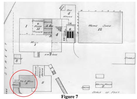
Detail from plan of *Geneva Worsted Mill, Heaton & Cowing Mill Co.*, Barlow's Insurance Survey No. 9758 (1889), showing continued use of the Heaton & Cowing Mill as Geneva's No. 2 Mill (A, circled) and its wheelhouse, as well as continued use of the Engine House, and the rear frame addition as a Dryer House (B).
