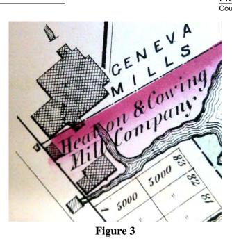
Detail from G.M. Hopkins, *Atlas of Providence RI* (1875) showing former headrace of the Heaton & Cowing Mill as adapted for the Geneva Mills. By this time, overflow from the main flow of the river had been rerouted to enter the Heaton & Cowing Mill's wheelhouse from Geneva Pond (not shown) to the west.
