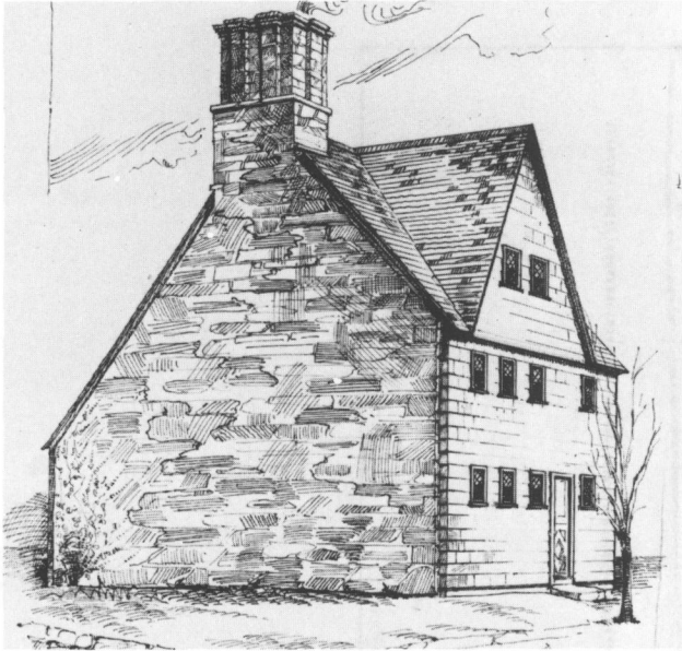
Fig. 1: Great Road (c. 1687): Norman M. Isham's drawing of a late-seventeenth-century "stone-ender," with widened plan.
