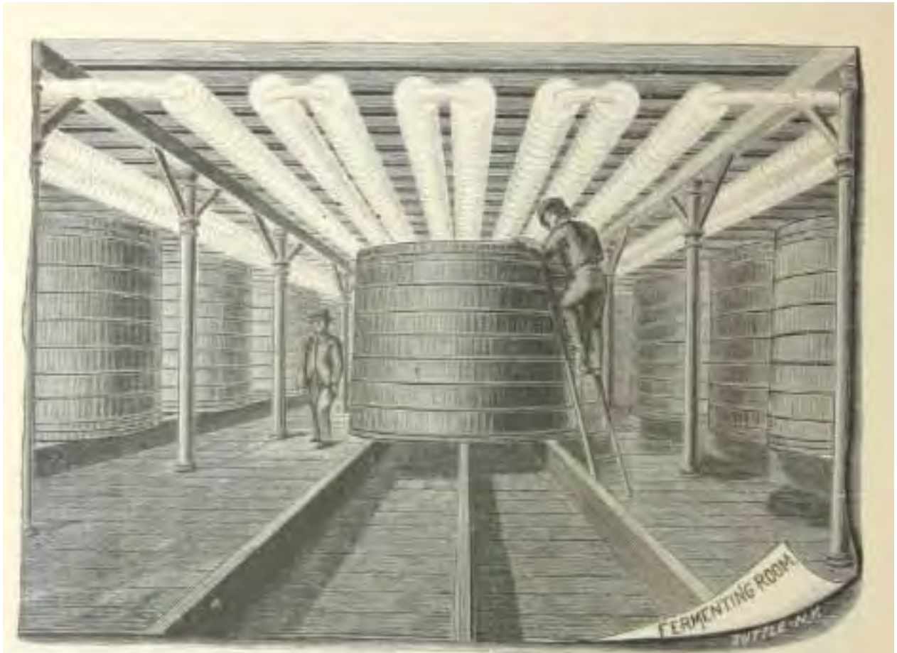
Figure 6 Fermenting Room showing arrangement of vats and cooling apparatus Illustration from De LaVergne Refrigeration Machine Co. catalog (1896)
