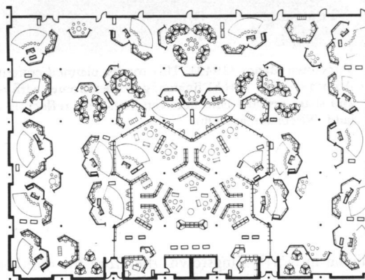
Fig. 81: Floor plan of the Great Room, North Kingstown High School addition (1970); 100 Fairway; Providence Partnership, architect. This design won national recognition for flexible planning in 1970.
